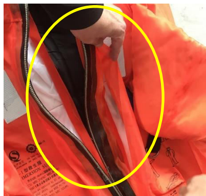
Figure 1: Immersion suit zippers were found defective.
