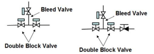
6.3.2.4 Examples of appropriate isolation arrangements are shown below. Isolation arrangements are to be fitted on the exposed deck in the hazardous area. Also, ballast water originating from a hazardous area is not to discharge into a non-hazardous area, except as given in 6.3.1.7.
