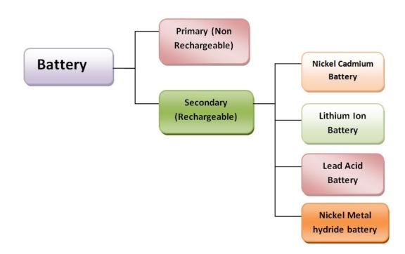
1.4.2 Lead acid, Ni-Cd batteries are extensively used for various ship board applications. Over the years, Lithium ion batteries have started replacing other type of batteries in maritime installations due to their high energy density. Lithium-ion is named for its active materials; the words are either written in full or shortened by their chemical symbols. Battery chemistries are generally identified in abbreviated letters.
