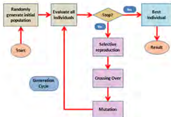
Figure1: Flow Chart of Genetic Algorithm Generation Cycle
